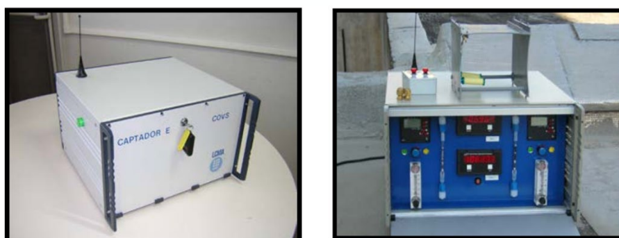
Figure 2. VOC capture system. Source: UPC (2019)
